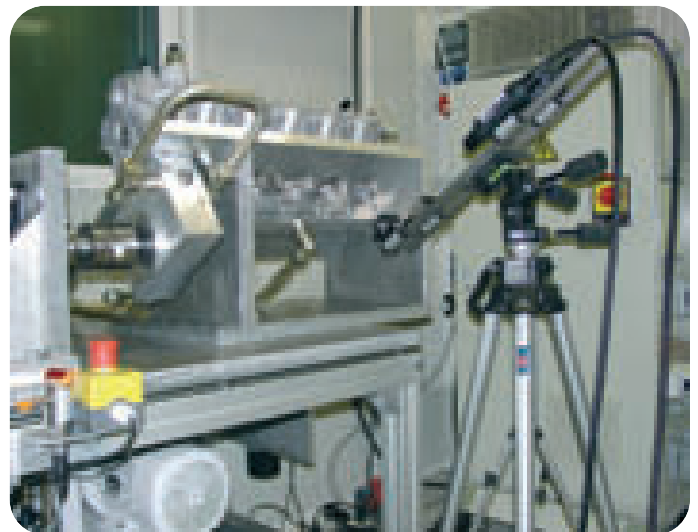
Figure 1 Test bench with Porsche Carrera GT cylinder head and non-contact laser measuring system
