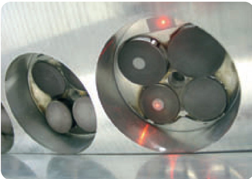
Figure 2 Valve head and reference point with laser beam for differential measurement
