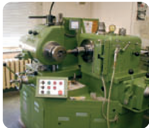
Figure 1 The machine before any modifications were carried out. The photo shows the input and output spindles and the location of the hand-brake on the output side.
