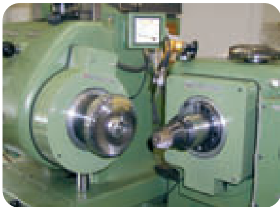
Figure 4 Microphone positioned above gearset mounted on input and output spindles.
