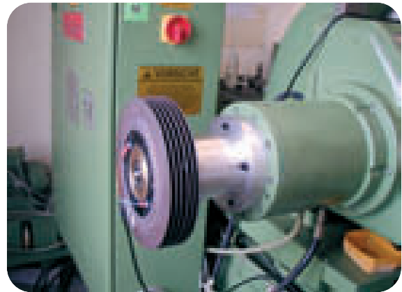
Figure 5 Magnetic particle brake assembly.
